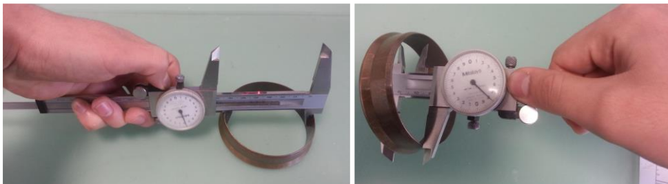
Fig. 4.11: Measuring the interior dimensions of the mould
