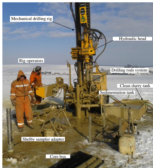
Fig. 12.6: Mechanical drilling (wire line)
